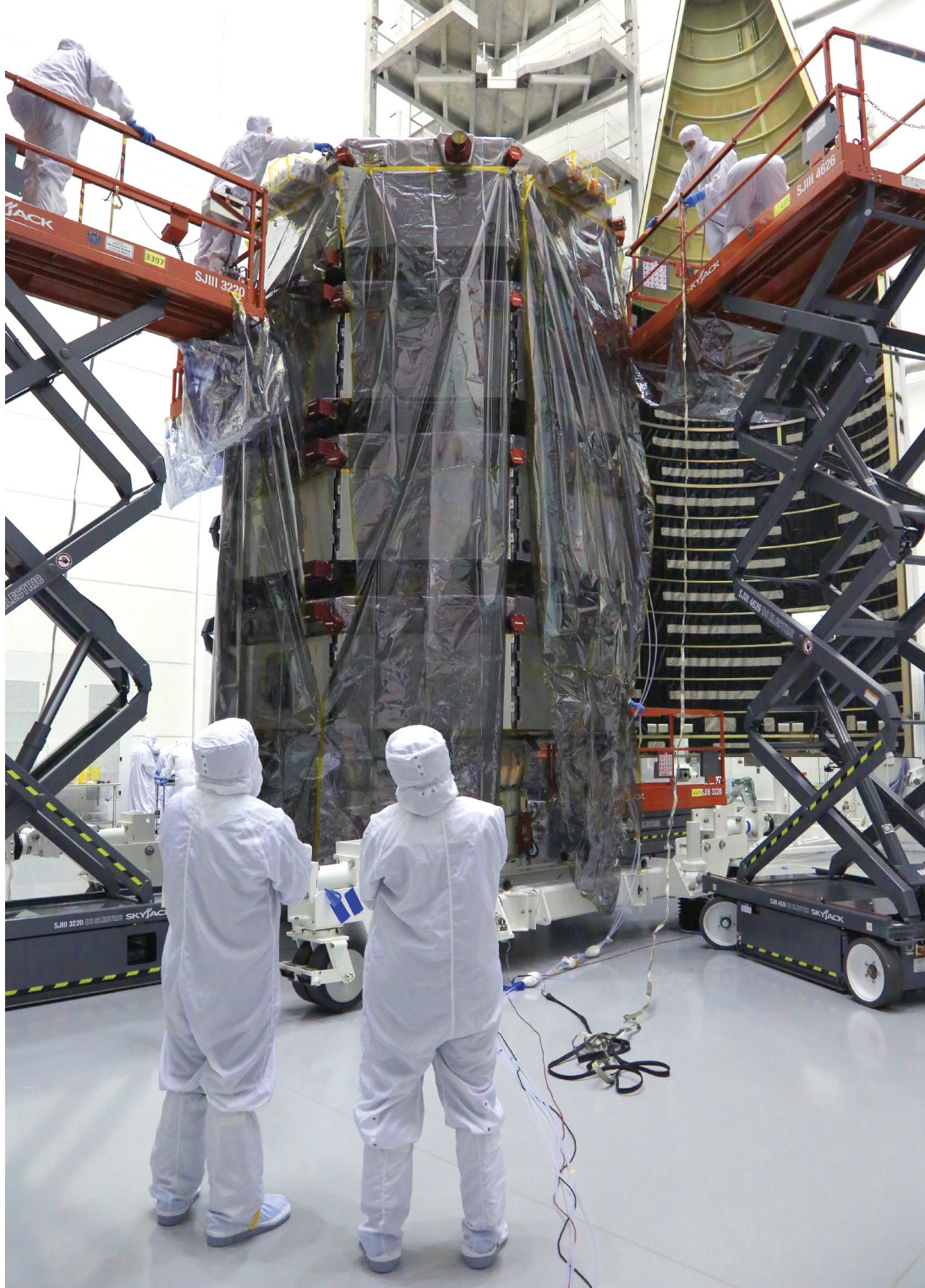
Each of the four MMS observatories is octagonal in shape, approximately 11 feet across by 4 feet high. When stacked together inside the Atlas V launch vehicle, the observatories are more than 16 feet tall.
