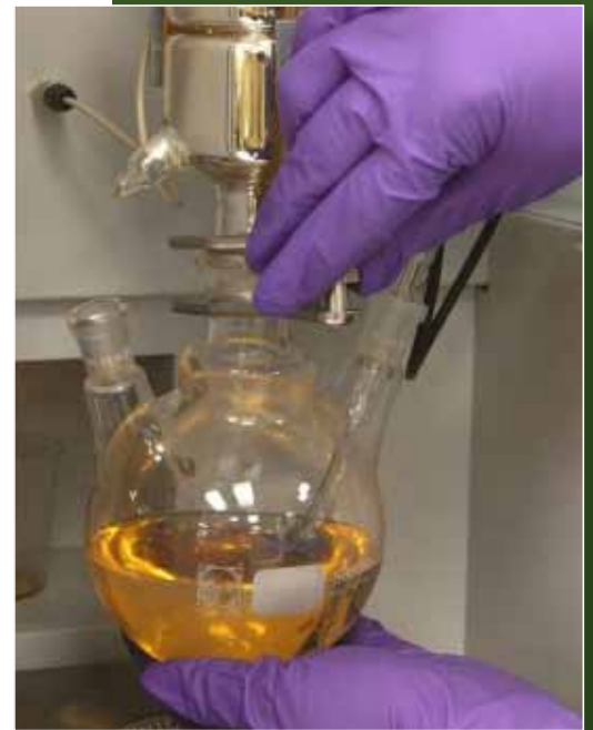
Vacuum distillation test for biodiesel samples
