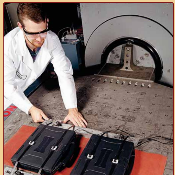
Equipment is exposed to simulated vibration and shock on electrodynamic shakers for evaluation of performance during transport and operation.
